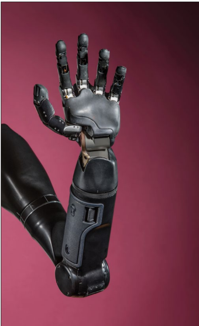
A modular prosthetic limb with more than 100 sensors.
