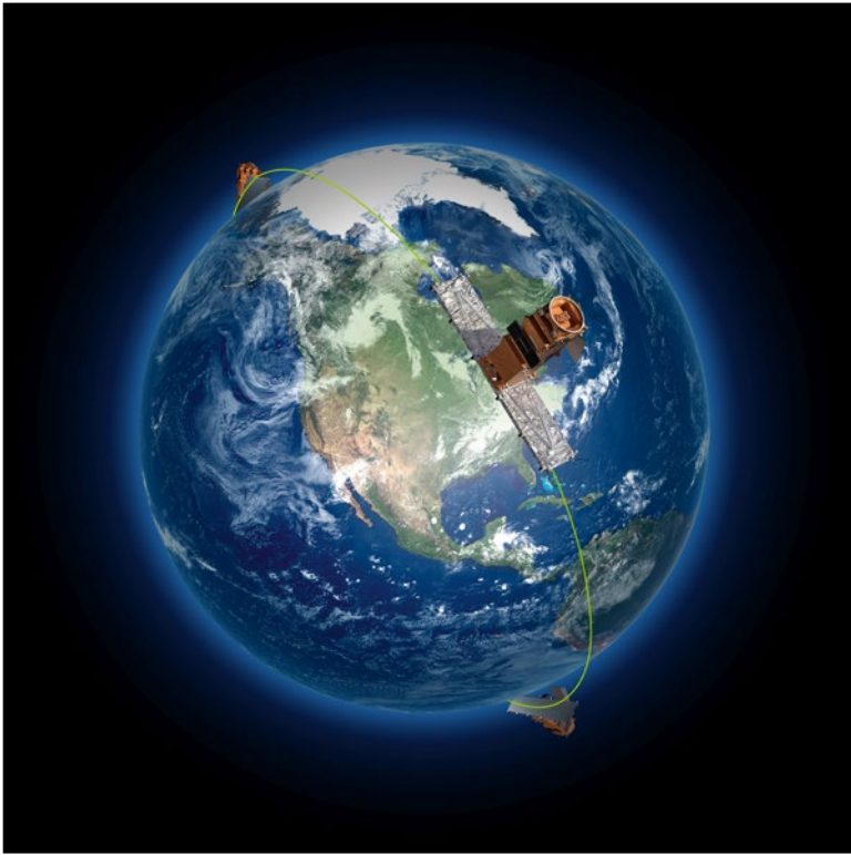
The three RADARSAT Constellation Mission spacecraft will be evenly spaced on the same orbital plane at an altitude of 600 kilometres.
