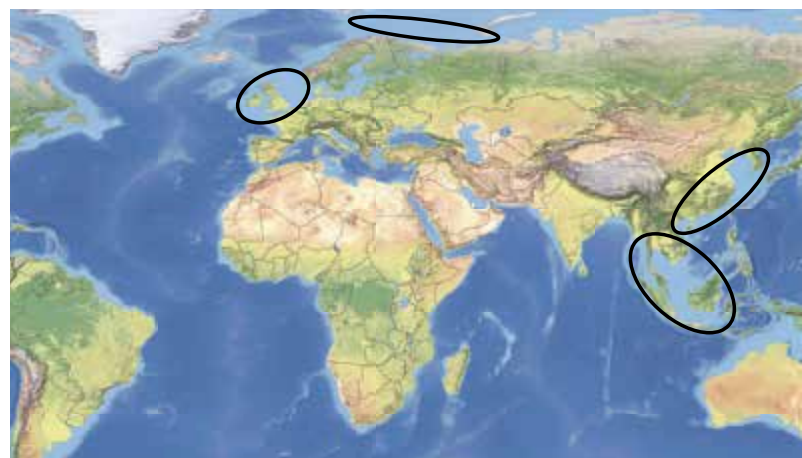
Shallow water, depicted in light blue, results in poor hydroacoustic conditions for ASW forces due to multipath propagation for passive sonar and high levels of bottom reverberation for active sonar. (Based on National Oceanic and Atmospheric Administration map, adapted by CNAS.)
