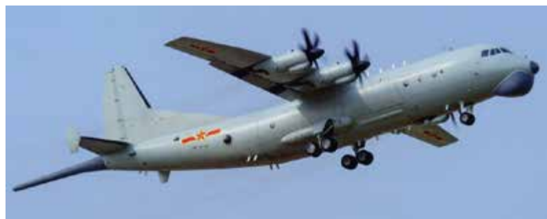
Chinese People's Liberation Army Navy Air Force Y-8 maritime patrol aircraft carries maritime search radar under the nose, electro-optical/infrared turret aft of the nose landing gear, weapons bay forward of the main landing gear, and magnetic anomaly detector boom aft of the tail. (PLARealTalk.com)
