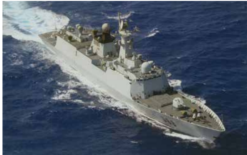
Chinese People's Liberation Army Navy (PLAN) Type 054A Jiangkai II-class frigate represents a significant ASW capability improvement for the PLAN through the integration of a variable depth sonar and a hangar to support the embarkation of an anti-submarine warfare helicopter such as the Z-9 helicopter on the stern in this photo. (Chinese Military Review)
