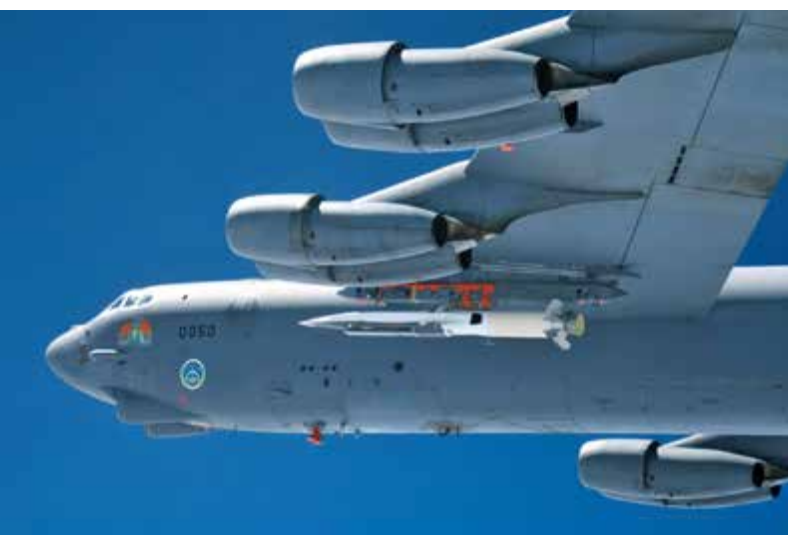
A B-52H Stratofortress, loaded with an X-51 experimental hypersonic weapon, epitomizes the ability of some weapons systems to adapt to new challenges. (U.S. Air Force)
