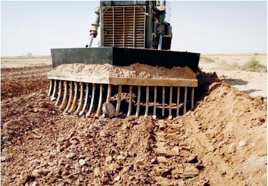
A locally developed demining tool that is installed in front of a bulldozer in Iran
